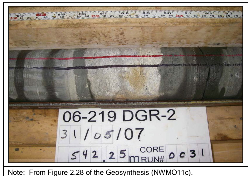
Figure 4-11: Core Sample of Interbedded Shale and Limestone, Georgian Bay Formation, 542.25 mBGS, DGR-2
