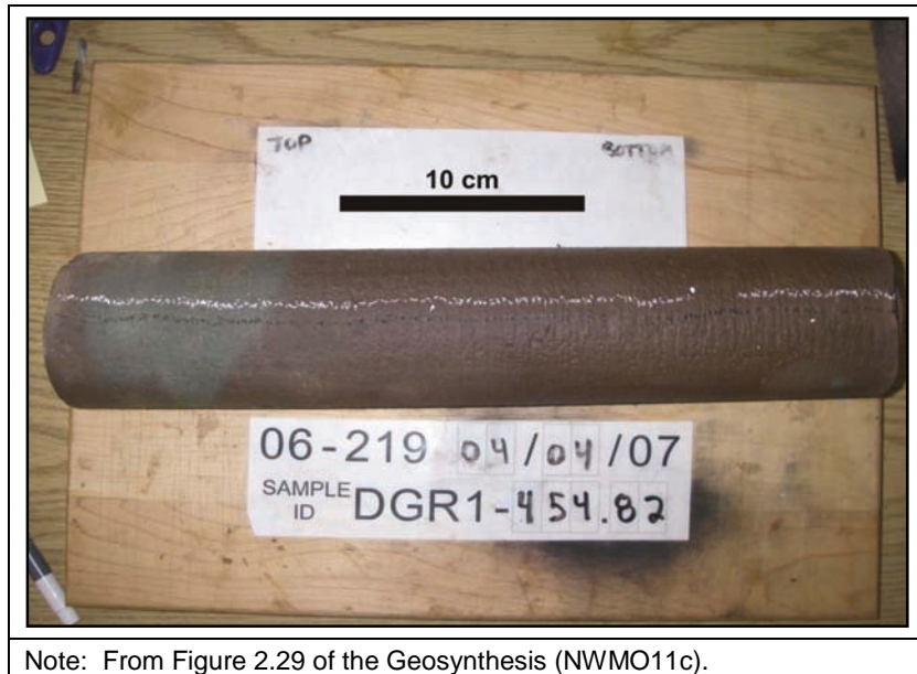
Figure 4-10: Core Sample of Green and Red Calcareous Shale, Upper Ordovician Queenston Formation, 454.82 mBGS, DGR-1
